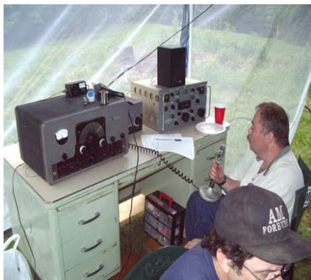
John KB1FQG Running a 200+ pound (not including the desk) Plate modulated AM Classic station.
