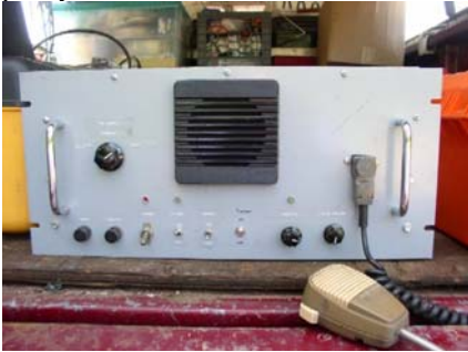
Figure 1 - New 2M repeater assembled by WA1HUD, sitting in the back of Steve's truck just before installation. The main ingredient is a GE Master II repeater.
