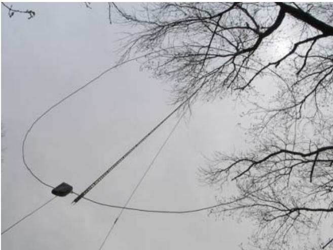
The 15 foot by 3/8" loop. Note coax feed going to top, and tuning cap at bottom.
