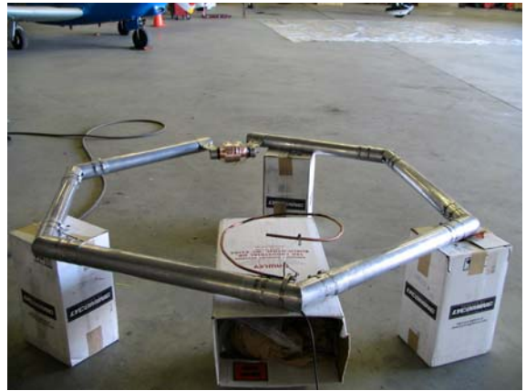
Half size version of the “earring” on the test stand showing tuning loop and capacitor
