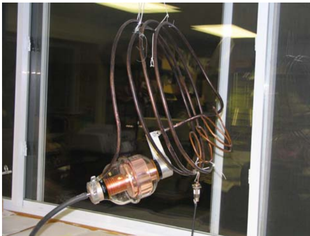
Four turn receiving loop with the big 1000-20 pf Soviet capacitor
