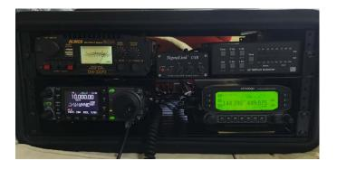
I built this box to make field day and camping trip well organized. This unit can run on 110 volt power from the grid or from my 200 watt Honda generator. It can also run on a 12 volt deep cycle battery if needed.
