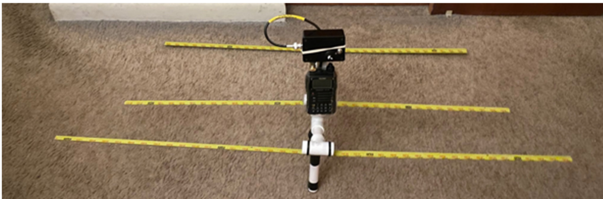
K1MJC's tape measure Yagi
