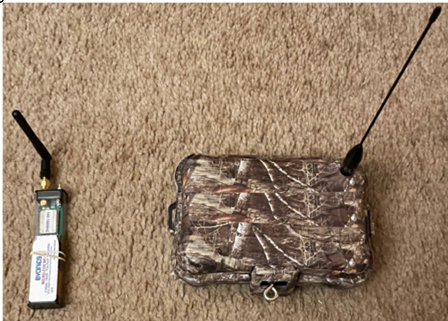
Byonics MicroFox 15 (left) and its custom armor (right).
